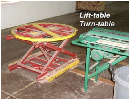
lift table reduces bending load
